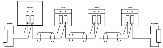
There must be no more than two wires connected to each terminal, this ensures that a "Daisy Chain or "straight line" configuration is used. A "Star" or a network with "Stubs (Tees)" is not recommended as reflections within the cable may result in data corruption.
